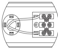
6. Plug the grounding wire on the cover plate into the casing as shown.
