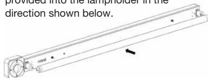
9. Then rotate the lamp 90° to secure it in place.
