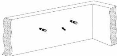
4. Mount the fixture on the wall or ceiling, aligning the mounting holes to the wall anchors and securing with the anchoring screws.
